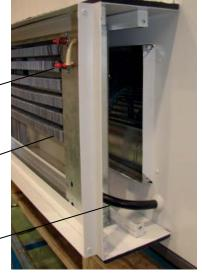
Then, unscrew the screw that fastens the electrical heaters' frame and take out by the rail, as shown in the following images.
