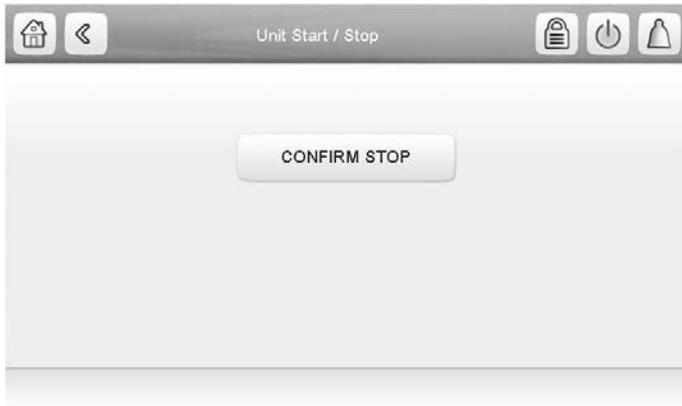
Confirm the unit shutdown by pressing **Confirm Stop** or return to the previous screen by pressing the **Back** button
