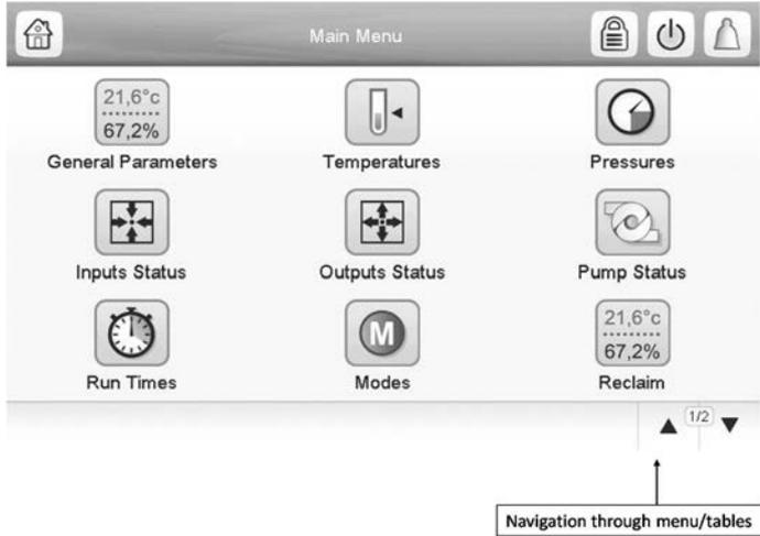
Specific unit parameters table/menu can be accessed by pressing the icon corresponding to the desired category. In order to go back to the Synoptic screen, press
