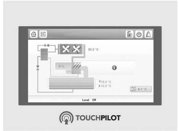
The bell located in the upper-right part of the screen lights when any fault is detected (see also section 8.2).
